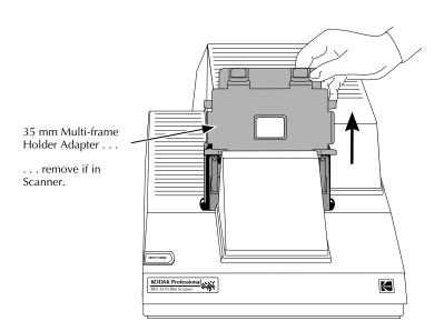
B. If a single-frame film holder is in the Scanner, remove it.
